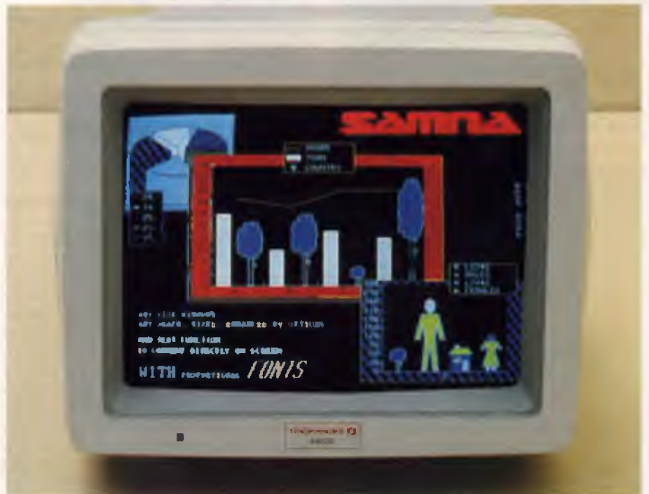
Figure 3. In EGA mode, the Thompson 4470D monitor offers the same resolution as the Multisync, as well as four text colours.
