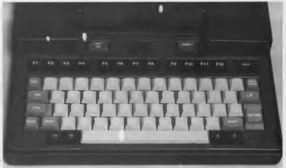
Figure 1. The 73 keys include 12 function keys (which can be shifted), a large Help key, Reset, Line Feed, Return, Tab, Control, Backspace, Escape, Shift and Shift Lock.
