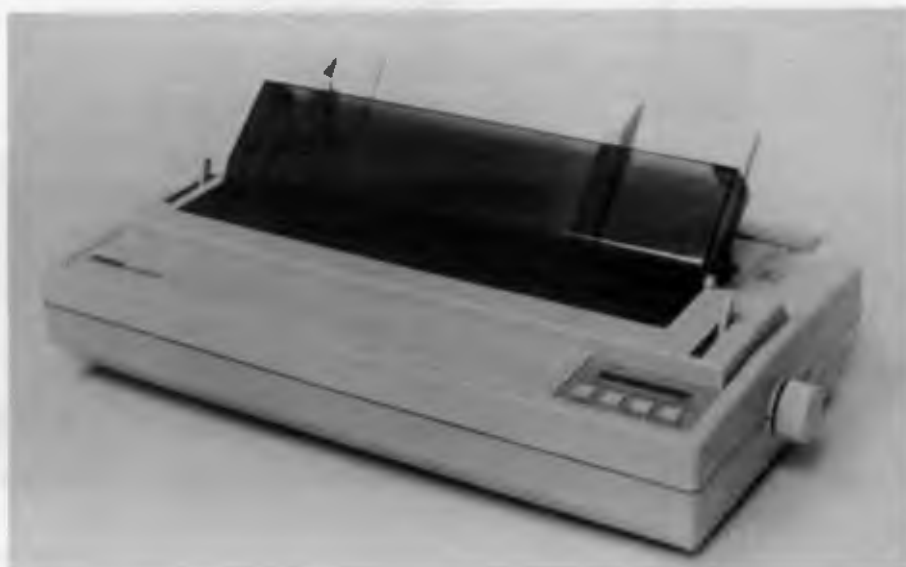
The 24-pin Epson LQ 2500+. The control panel allows access to many of the printer's settings, and can be used to set macros.
