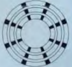
Figure 1* Perfectly aligned tracks. The black areas are "read only." These store critical track and sector ID information. The white areas are data sectors and store your system, programs and data.
